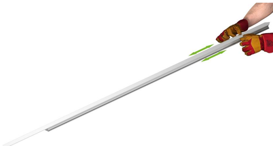
Fig. 5.28: Clamp on cover strip approx. 3 cm
